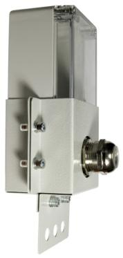
Besides the measurements of the distance to the available mobile devices of the system, RealTrac Access Point acts as repeater while data transmitting from any other access points to the RealTrac System's server and backwards.
